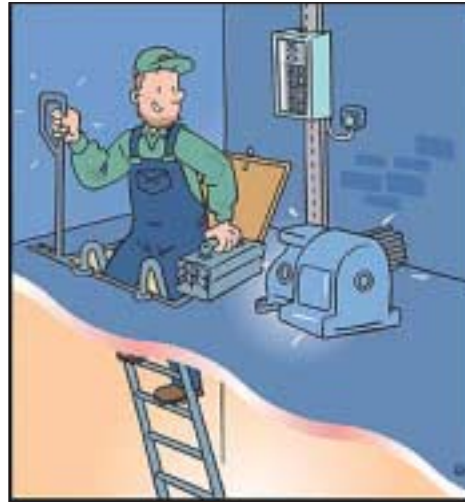
Install the necessary ladder, handrail & equipment for a safe and easy access to the machine room
